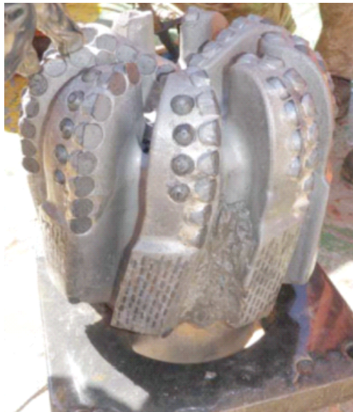
Figure 6. Hybrid PDC-Impreg Bit Used to Drill Hard Carbonate Formation Deepwater Canada
