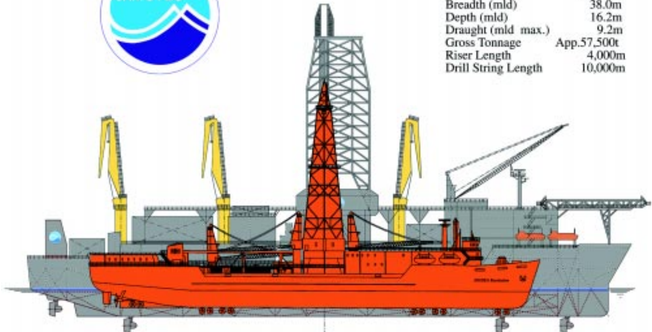
Figure 37. Silhouettes of ships representing the two primary drilling platforms to be used in the IODP. In the foreground is a silhouette of the JOIDES Resolution . A comparable ship, with enhanced capabilities, will be part of the new program. In the background is the present general design of a deep-water riser drilling ship produced by JAMSTEC in consultation with the international community. General design specifications for this new ship are shown in the upper right corner. Detailed design of this ship has been completed and construction began in 2000.
